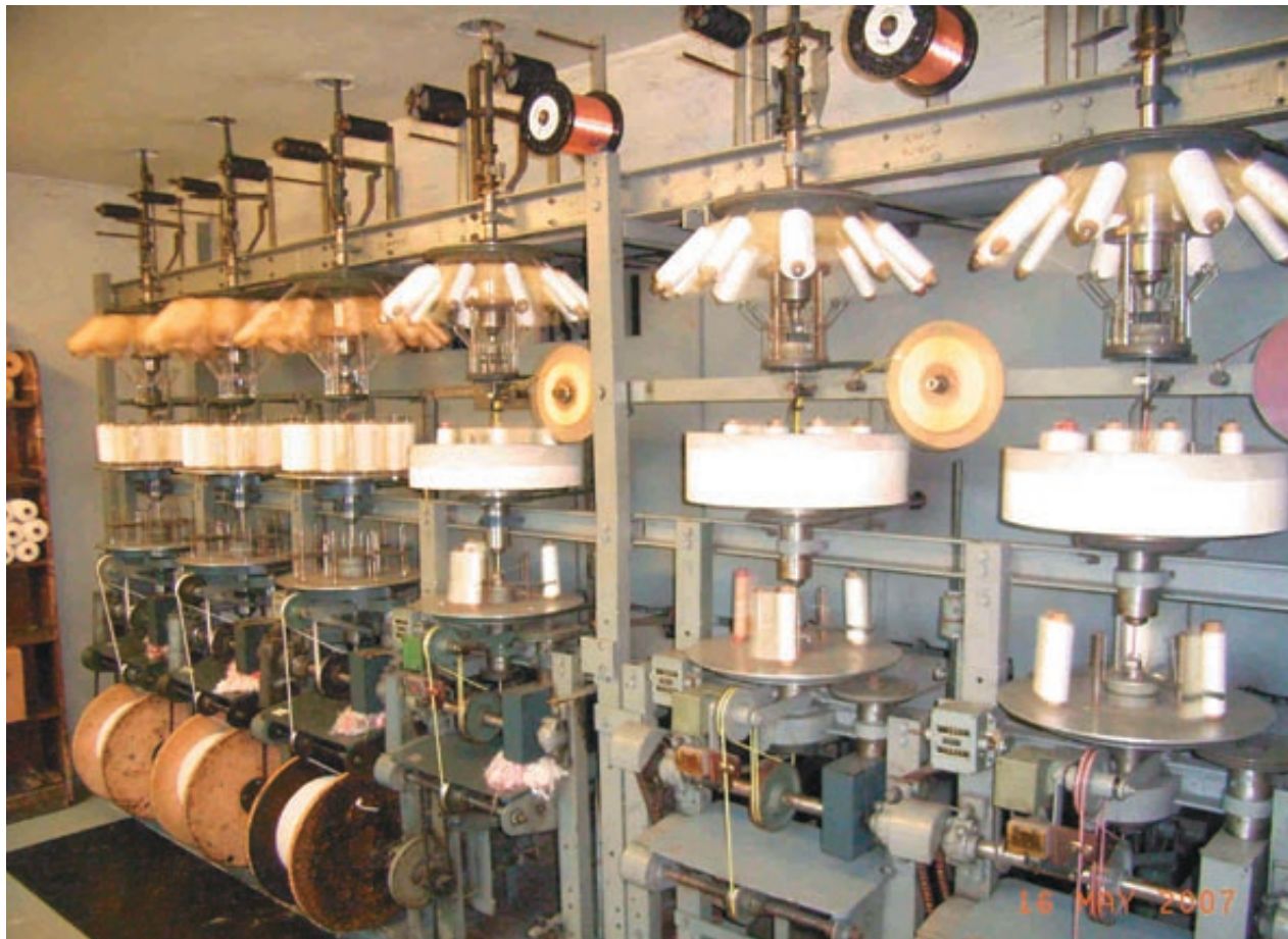
Fuse winding machines in action. Photo courtesy of WANO Schwarzpulver GmbH
